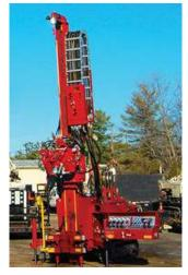
Drill rig used to collect soil
